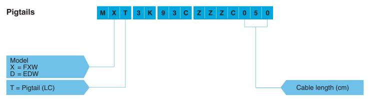
MXT.3K.93C.ZZZC050 = 1 FXW plug (key W), 3K.93C series and one pigtail (LC) on the other side, 50 cm length.
